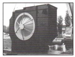
**Centrifugal Fans** • relatively low pressure air supply or exhaust and fume exhaust fans in industrial applications where there are low levels of particulate matter in the air stream. Can operate at temperatures up to 600 °F.
